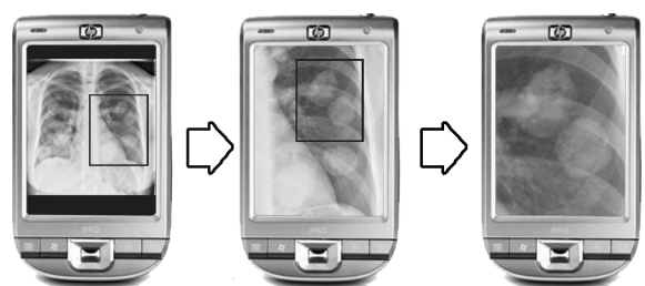
Figure 6. JPEG2000 streaming to handheld device - from low resolution version of medical image to region of the image in original resolution
