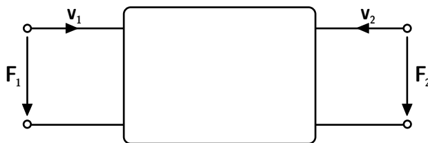
Fig. 10.16. Mechanical two-port, analogy I (force/voltage)
