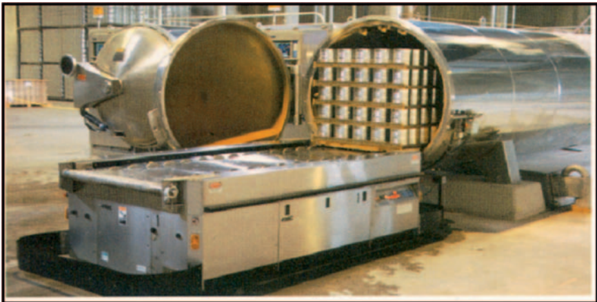
FIGURE 9.5. Automated guided vehicle for batch retort loading/unloading (Courtesy, FMC Food Tech., Madera, CA).
