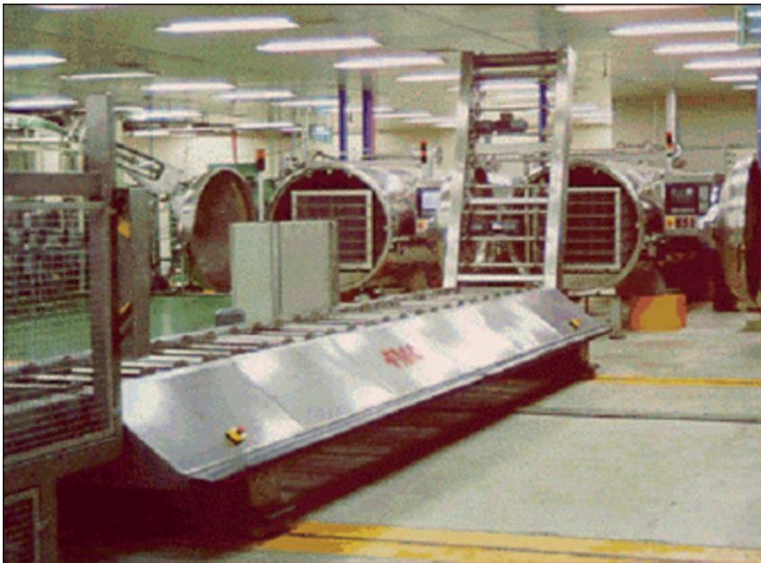
FIGURE 9.8. FMC shuttle system for automated batch retort loading/unloading (Courtesy, FMC Food Tech., Madera, CA).
