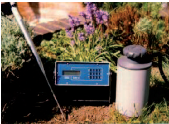
FIGURE C Soil respiration system that SRC-1 connected with EGM (left) and CIRAS (right) from PP Systems.
