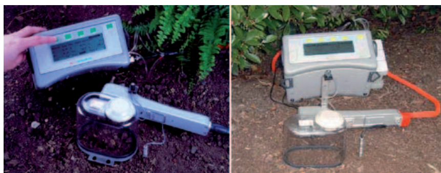
FIGURE E The measurement of soil respiration in the field by SRS1000 Ultra compact soil flux system (left) and SRS2000 Intelligent portable soil flux system (right).
