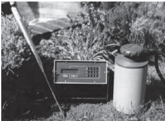
FIGURE C Soil respiration system that SRC-1 connected with EGM (left) and CIRAS (right) from PP Systems. (see color insert in back of the book)
