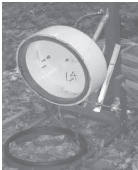
FIGURE G Automated soil respiration chamber in the open position. (see color insert in back of the book)
