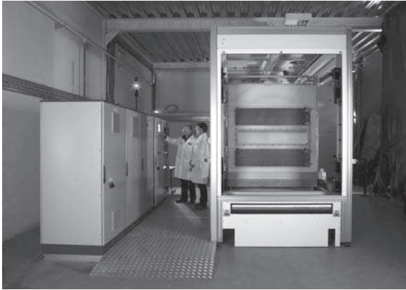
4.14 The Dow Corning Plasma Solutions SE-1000 AP4 large area web processing system showing front view of vertical electrode and control cabinets. (Courtesy of Dow Corning Plasma Solutions 2 .)
