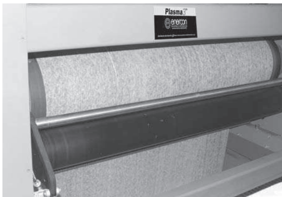
4.17 A nonwoven under APP processing by Enercon's Plasma3™ system. (Courtesy of Enercon Industries Corporation 3 .)
