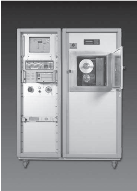
3.3 Roll cassette for the plasma treatment of small width webs in a classical box-shaped vacuum plasma system.
