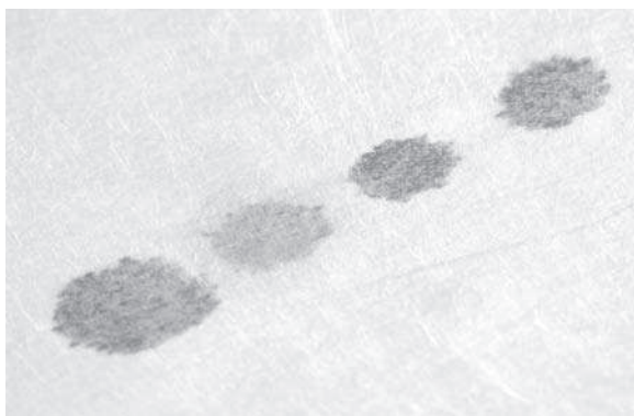
3.6 Illustration of wettability of meltblown nonwoven PP, coated with a permanently hydrophilic coating.
