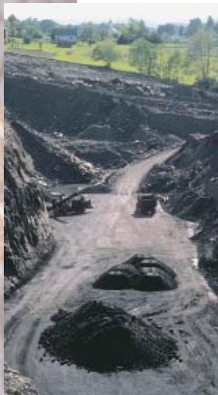
Mining for coal at this site in Pennsylvania is done using the “strip mining” method. This technique physically moves the soil back from the coal bed. Strip mining causes at least a temporary elimination of the native animals’ habitat.
