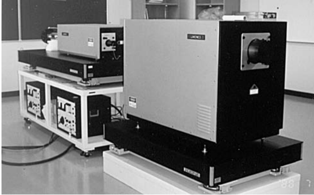
Figure 3.10. An example of a commercially available TEA-CO 2 laser (Lumonics).
