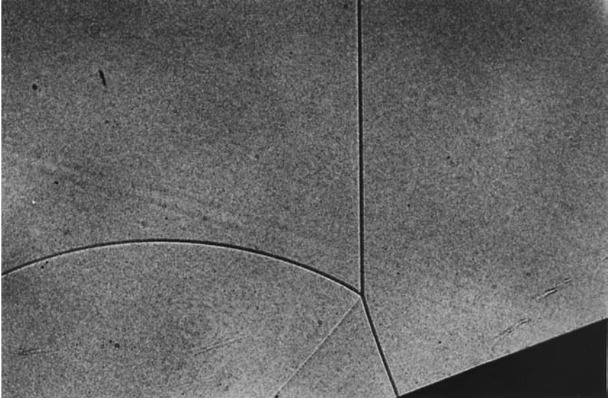
Figure 6.4. Image of a shock wave obtained using shadowgraphy [2]. The shock wave originated to the left of the figure, and propagated from left to right. The flow in the region in the lower side has a complicated structure. (Photograph courtesy of Professor K Matsuo, Kyushu University.)
