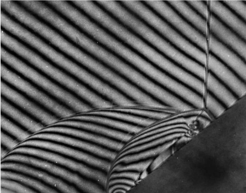
Figure 6.5. Photographic image of a shock wave obtained using an interferometric method [3]. The laser apparatus used for the measurement was the same as that for the image shown in figure 6.4. (Photograph courtesy of Professor K Matsuo, Kyushu University.)
