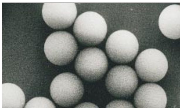
Fig. 15. Light microscope photograph of SOURCE. Note the uniform size distribution and absence of broken beads and bead fragments.
