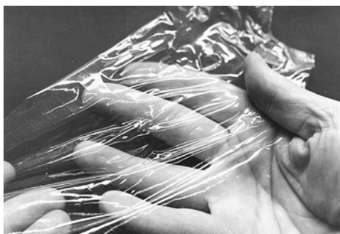
Figure 3.13 A thin film of poly[ bis (butyl-amino)phosphazene] fabricated by solution casting for membrane experiments.
