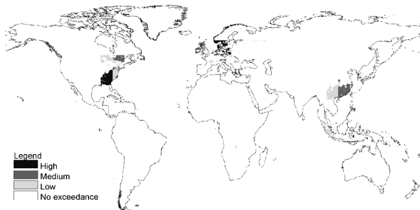
Figure 17 Estimated exceedance of critical loads (applied to the sensitivity map – Figure 8) by 1990 sulfur deposition estimates minus neutralizing base cation deposition derived from soil dust. (Exceedance scale in \text{meq m}^{-2} \text{yr}^{-1} : low 0–50; medium 50–100; high > 100 ) 41
