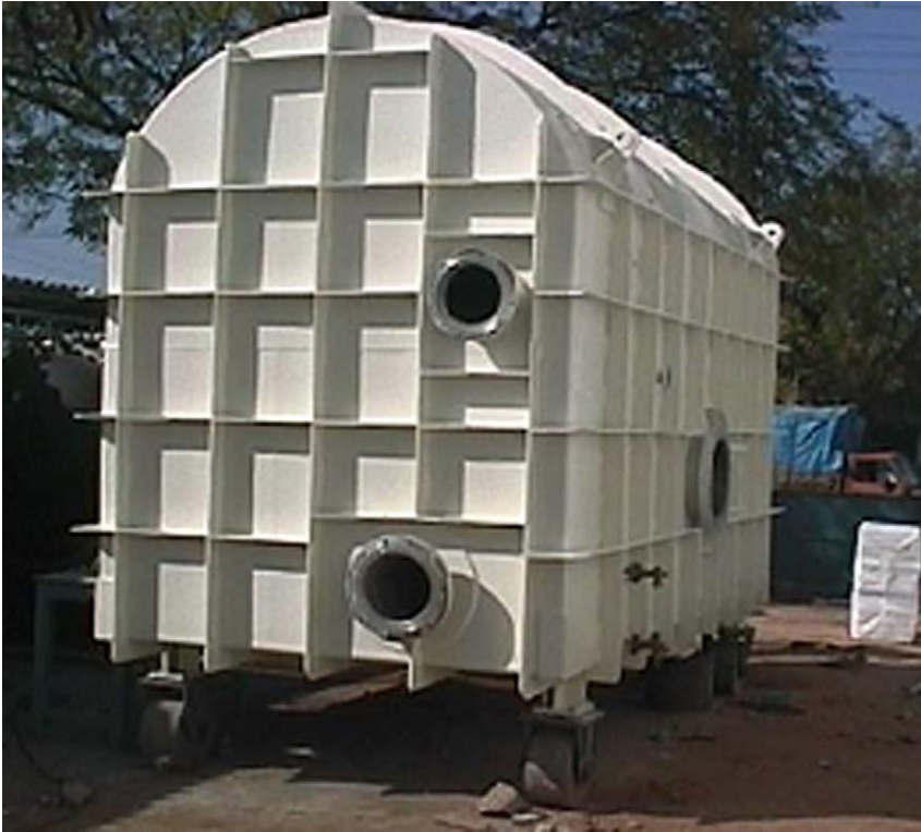
Fig. 9.7. A view of the flash chamber at the Kavaratti LTTD plant.
