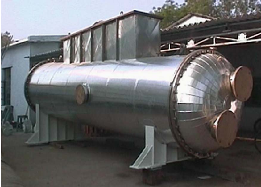
Fig. 9.8. A view of the cylindrical condenser in operation at the Kavaratti LTTD plant.
