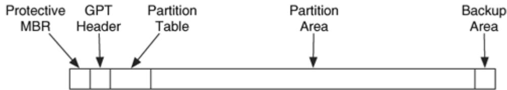
The second part of the GPT disk starts in sector 1 and contains the GPT header. The header defines the size and location of the partition table, which are fixed when the GPT disk is created. Windows limits the number of entries in the partition table to 128 [Microsoft 2004]. The header also contains a checksum of the header and the partition table so that errors or modifications can be detected.
