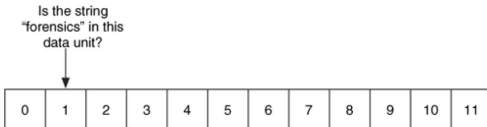
This search technique has historically been called a physical search because it used the physical ordering of the sectors, but I do not feel this is accurate. This was accurate when a single disk was being analyzed, but this is not true for systems that use disk spanning and RAID. For those systems, the order of the sectors is not the physical order, and a more precise name should be used.
