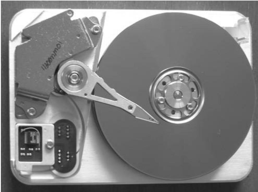
Inside the disk is an arm that moves back and forth, and it has a head on the top and bottom of each platter that can read and write data, although only one head can read or write at a time.
