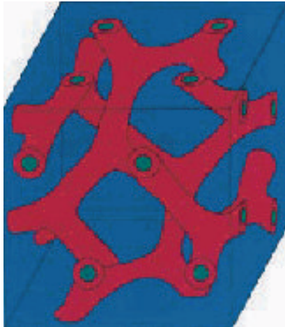
Figure 19.9. Schematic representation of the core-in-shell gyroid morphology found in the poly(isoprene- b -styrene- b -dimethylsiloxane) (ISD) triblock copolymer ( f_{PI} = 0.40 , f_{PS} = 0.41 , f_{PDMS} = 0.19 ). Blue, red, and green regions correspond to I, S, and D domains, respectively (adapted by Shefelbine 1999).
