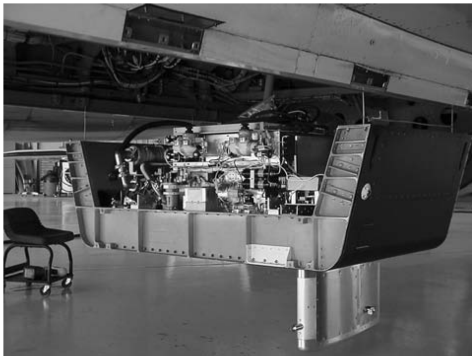
Figure 7.5 Photograph of an automated NO-NO y instrument mounted in a lower-fuselage pallet (1 of 4) on the NASA WB-57F. The instrument is hoisted into position so that the pallet forms the lower fuselage skin. The heated sample inlet extends below the pallet. (Photo courtesy of David J. Knapp.)
