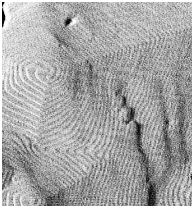
Fig. 4. AFM deflection image of the Cu(111) surface during deposition of copper. The steps are one atom in height. In the upper left are two nested spiral terraces.
