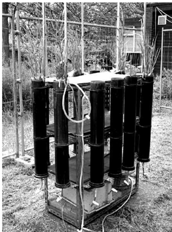
Fig. 26.1 Constructed treatment wetland rig (The King's Buildings campus; The University of Edinburgh) in May 2004.
