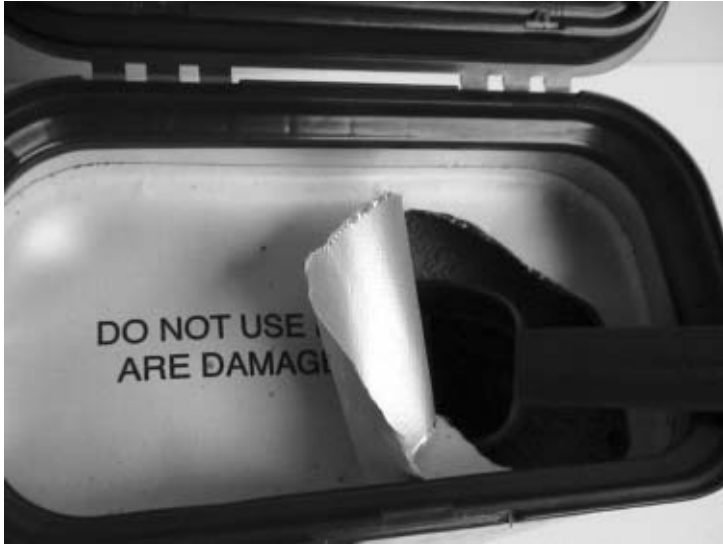
Figure 7.14 Container with over-cap and diaphragm seal broken.
