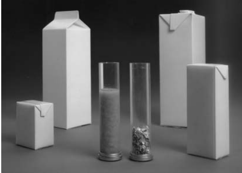
Figure 5.29 Liquid cartons – recovery of components.
