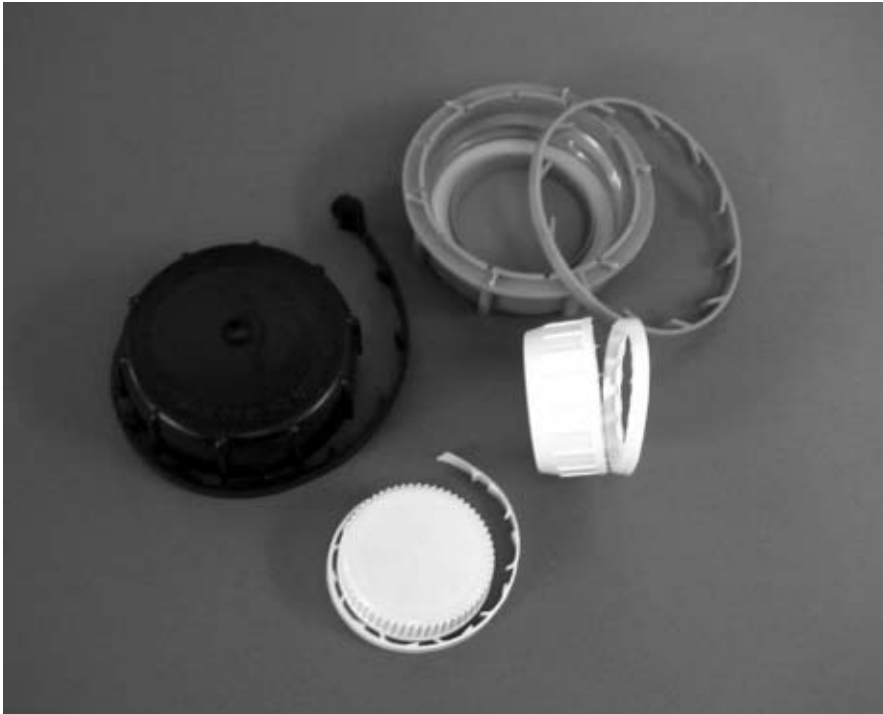
Figure 6.21 A selection of tamper-evident plastic closures. Clockwise from top right: Large closure with 'break-free' pawl-type tamper ring, shown after removal; Small closure with post-moulding blade-cut 'break-free' captive-type tamper ring, shown partially removed; Lightweight closure with 'pull-tab' pawl-type tamper ring, shown partially removed; Large closure with 'pull-tab' pawl-type tamper ring, shown partially removed.
