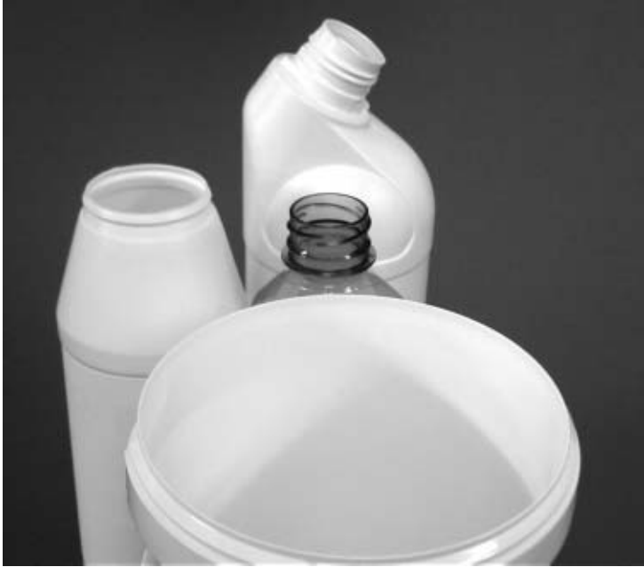
Figure 6.3 A selection of plastic container necks. Top – Extrusion blow-moulded, HDPE, modified butress-threaded, angled screw neck for child-resistant closure (CRC). Centre – Injection-blow-moulded, pre-formed PET, modified butress-threaded neck for tamper-evident capture bead sports closure. Left – Extrusion blow-moulded, spin-off trepanned wide neck with annular bead for push-on dispensing closure. Bottom – Injection-moulded, open top pail for press-on lid.
