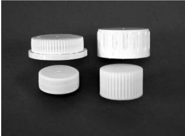
Figure 6.5 A selection of 'R3' and 'R4' plastic closures. Top left – 38-mm R3 shallow tamper-evident closure for HDPE fresh milk and juice bottles. Top right – 38-mm R4 deep plain closure for general and industrial use. Bottom left – 28-mm R3 shallow plain closure for general use. Bottom right – 28-mm R4 deep plain closure for general use.
