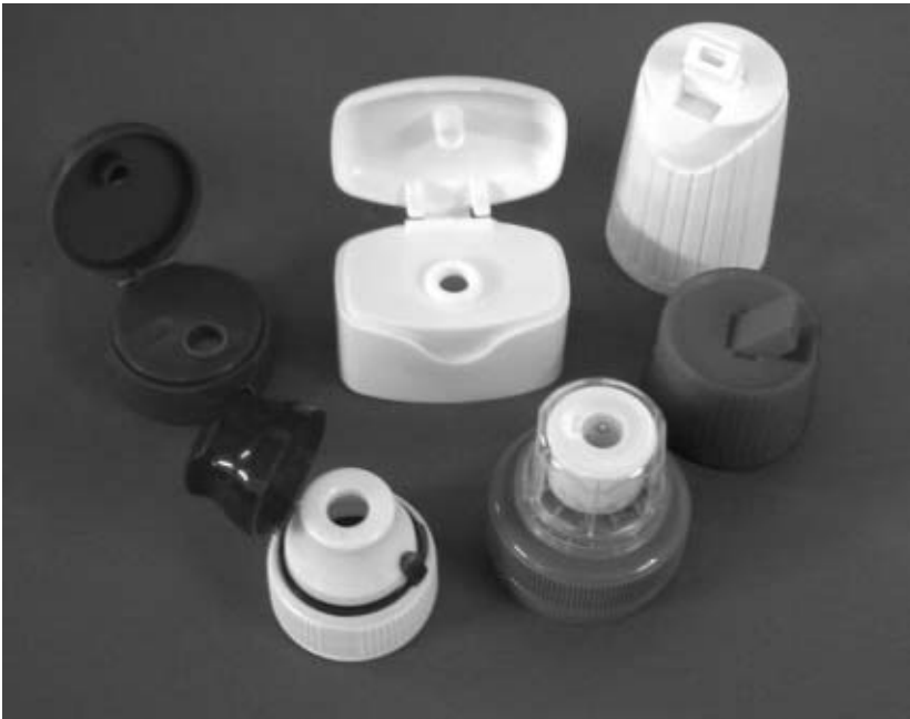
Figure 6.18 A selection of flip-top, directional nozzle and sports closures. Clockwise from top right: 28-mm tall closure with directional nozzle for household cream cleaner bottles; 28-mm closure with directional nozzle for household hygiene chemicals bottle; Sports closure with pull-up nozzle and tamper-evident overcap intact. Sports closure with pull-up nozzle shown with tamper-evident overcap raised. 30-mm closure with flip-top and induction heat-seal liner for squeezable sauce bottles; Press-on closure with flip-top for personal care products.
