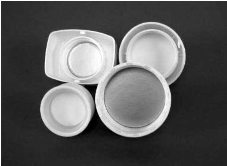
Figure 6.11 A selection of liner seal plastic closures. Top left – Press-on closure with induction heat-seal liner for personal care containers. Top right – ‘Squeeze-and-turn’ CRC with expanded polyethylene (EPE) liner for hazardous domestic chemicals containers. Bottom left – ‘Press-and-turn’ CRC with EPE liner. Bottom right – Heavy-duty plain closure with induction heat-seal liner for containers for agrochemicals.
