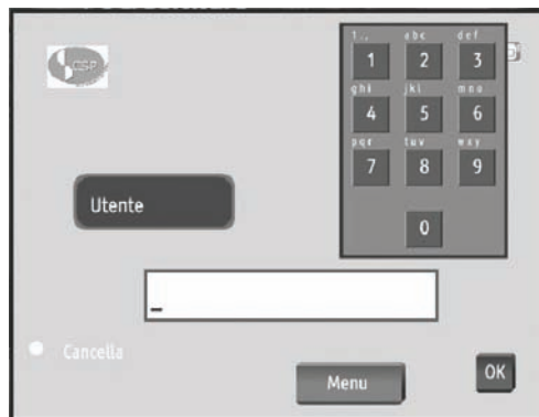
Figure 4. Multi-press with timeout and visual feedback keyboard
