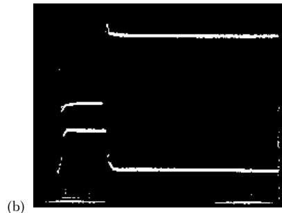
Figure 6.15 (a) Circuit used to pulse the MCT at 80 A. Note the 100 mΩ gate drive damping resistor. (b) Gate drive waveform; 10 V/div. vertical, 2 μs/div. horizontal (upper trace), voltage across 1 Ω load, 50 V/div. (lower trace)
