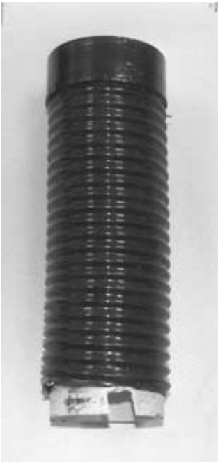
FIGURE 5-7. Bolt head clearance cutouts.
