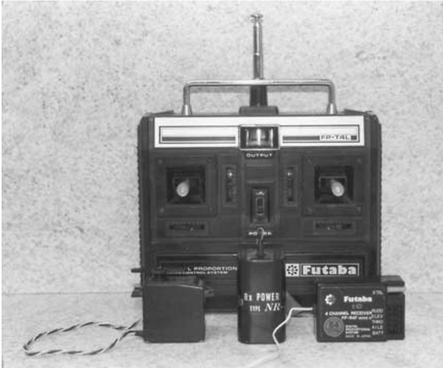
FIGURE I-15. Basic wireless remote control system.
