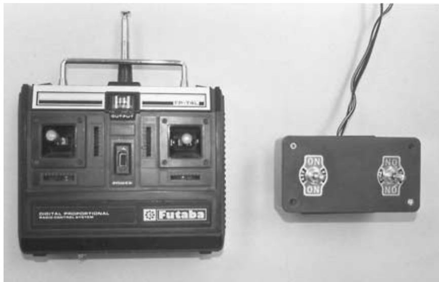
FIGURE I-14. Wireless and wired controls.
