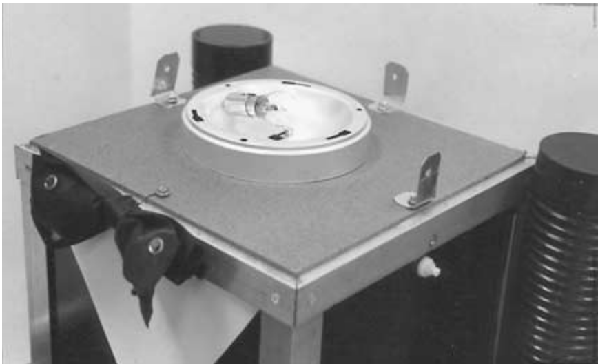
FIGURE 5-15. Mounting tabs for the head. Note the auto dome light in place.
