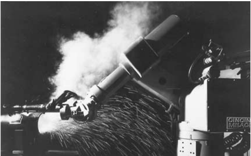
FIGURE I-4. Robots can do light work such as grinding. ( Courtesy of Cincinnati Milacron. )
