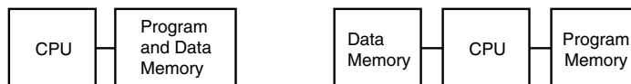
Figure 1-1: At left is the von Neumann architecture; at right is the Harvard architecture.
