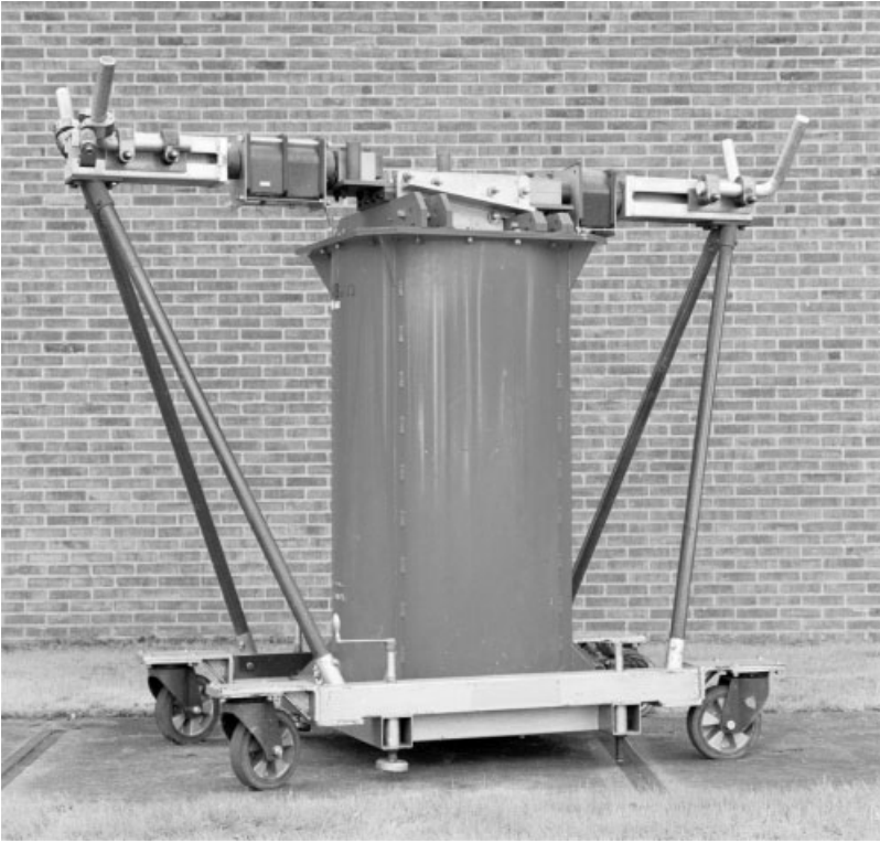
Figure 10.23 Coaxial shunt for measuring currents up to 100 kA rms with a bandwidth of 0–1 MHz (courtesy of KEMA)
