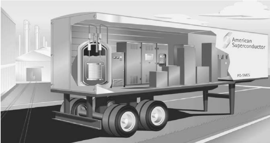
Figure 4.33 SMES cryostat and trailer. (Courtesy of American Superconductor.)
