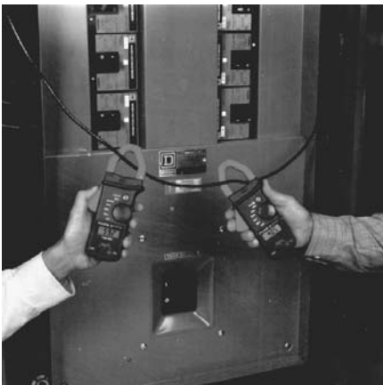
Figure 7.14 Average-responding rms to true rms ratio of less than 0.75. The meter on the left registers 59.2 and the meter on the right registers 40.5. (Reproduced with permission of Fluke Corp. ©.)
