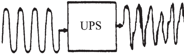
Figure 7.2 UPS distorted power.
