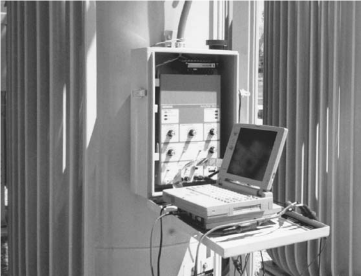
Figure 6.22 Flicker meter. (Courtesy of EPRI, PQTN Case No. 1, “Light Flicker Caused by Resistive Welder.”)
