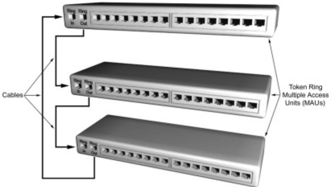
Figure 3.16 Construction of a token ring showing the cable connections in a three MAU ring.
