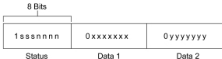
Figure 4.11 General structure of a MIDI message. The 8 bits are used to define the message type, the 4 bits are used to define the channel number, whilst the 0xxxxxx and 0yyyyyy bits carry message data. Source: Rumsey, Francis (1994) MIDI Systems and Control , Second Edition, Focal Press, p. 42.
