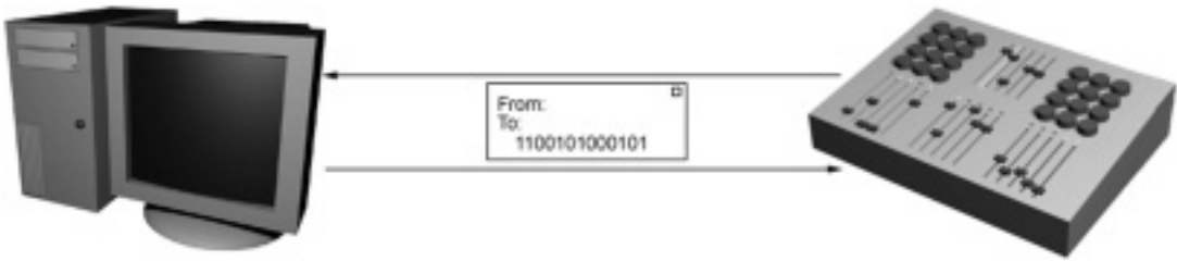
Figure 2.4 Point to point connections are generally described as connecting devices directly, as shown. In such a system, addressing information is redundant and not included, since there is only one other device from which the information can be sent.
