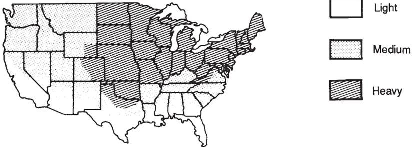
**Figure 2-7. Wind and ice load specifications.** Map shows territorial division of the United States with respect to wind and ice loading of overhead lines. Alaska is in the heavy zone and Hawaii is in the light. (*National Electric Safety Code*)
