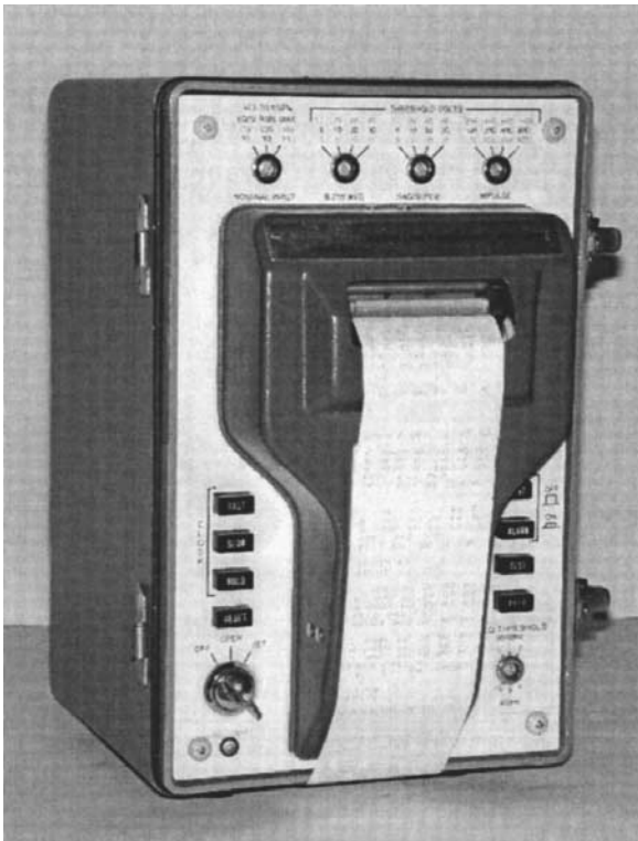
Figure 11.9 A first-generation power line disturbance monitor-analyzer, the Dranetz 606. (Courtesy of Dranetz-BMI.)
