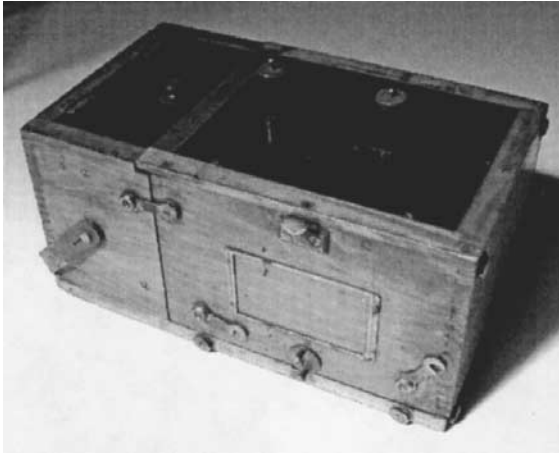
Figure 11.7 Early power quality instrument developed by GE in the 1920s to record lightning strikes. (Courtesy of Alex McEachern, from his personal collection of historical power instruments; www.Alex.McEachern.com .)
