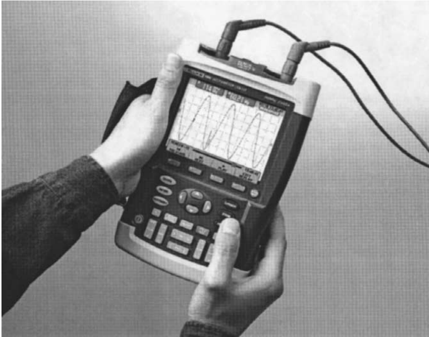
Figure 11.10 A hand-held oscillographic monitoring instrument. (Courtesy of Fluke Corporation.)
