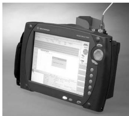
Figure 3.8. Example of a “platform” OTDR. [Credit: Agilent Technologies.]
