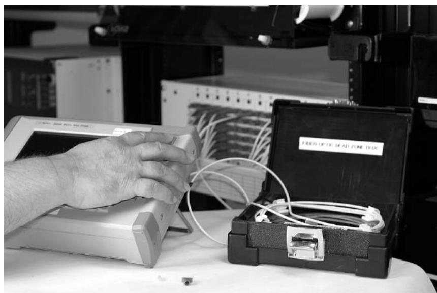
Figure 8.10. Single-mode fiber-optic dead zone box. [Credit: The Light Brigade.]
