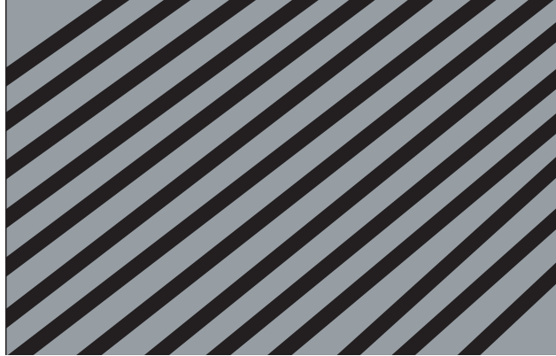
Figure 2.23. Interference pattern seen in a Michelson interferometer. The dark and light bands result from destructive and constructive interference. In this example, the mirror in one leg of the interferometer was tilted very slightly so that the recombining beams were not quite parallel and the difference in the path lengths of the two beams was much less than the coherence length. By increasing the difference in the two path lengths, the contrast between the dark and bright bands would be reduced. If the difference were much greater than the coherence length, the screen would be uniformly bright, without any interference fringes.
