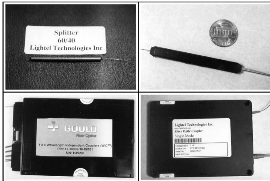
Figure 10.4 Examples of commercially available splitters. Clockwise from top left: 1-by-2, 1-by-32, 1-by-4, and 1-by-8 splitter. [Credit: The Light Brigade.]
