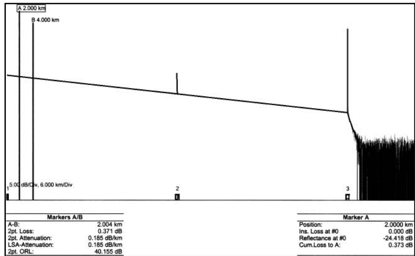
Figure 7.9. The OTDR trace of a mechanical splice is very similar to that of an APC (angled) fiber-optic connector. Both the APC and a mechanical splice with index-matching fluid or gel have ORL values of 50–60 dB.
