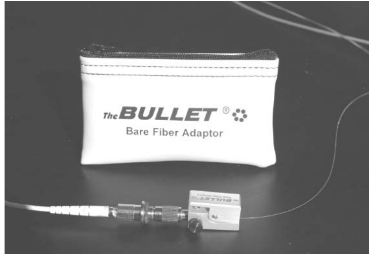
Figure 15.9. Bare fiber adaptor used at the end of a test jumper for accessing fibers. [Credit: The Light Brigade.]
