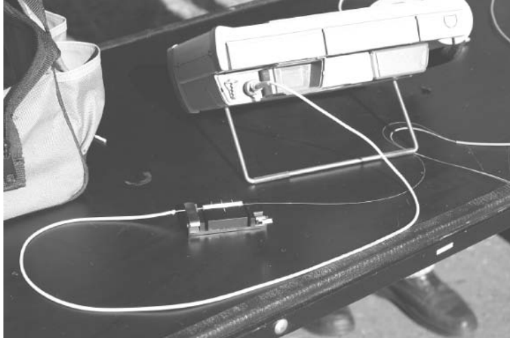
Figure 7.10. Reusable Norland UVC splice for testing unterminated optical fibers. [Credit: The Light Brigade.]
