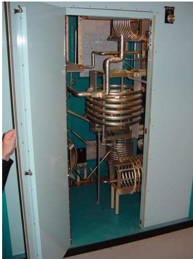
Figure 3.18: High power inductors formed from hollow tubes.
