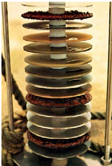
Figure 11.1 Corrosion test spool. (ref. 15).
