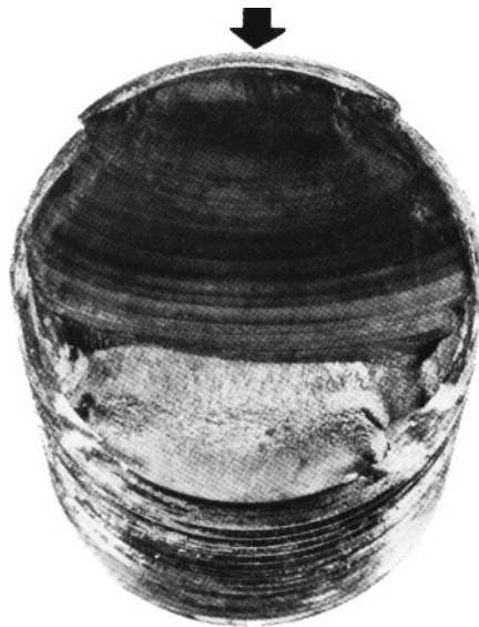
Figure 3.6 Metal fatigue fracture surface showing beach marks. (ref. 3).
