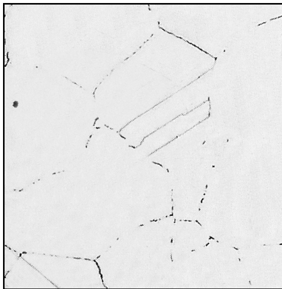
Figure 5.4 Intergranular corrosion of a sensitized stainless steel. (ref. 9).
