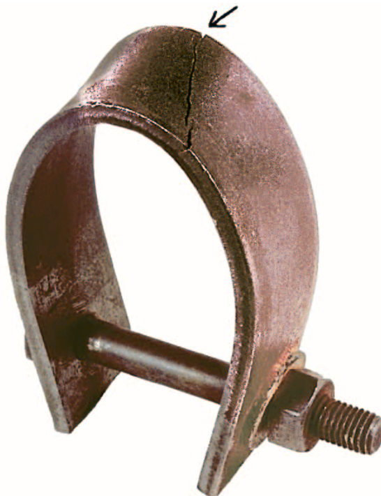
Figure 11.5 Typical U-bend test specimen with cracking showing danger of SCC. Carbon steel sample partly immersed in hot caustic solution was expected to crack readily and did, so that behavior of other metals could be compared.
