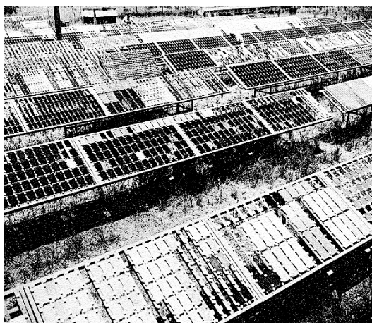
Figure 11.2 INCO test racks at Kuré Beach, NC. (ref. 16).
