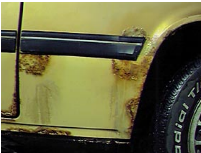
Figure 8.3 Automobile corroded by road salt.
