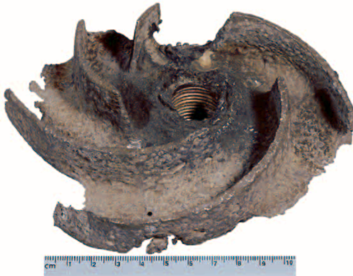
Figure 7.5 Cavitation of pump impeller in sour crude oil.
