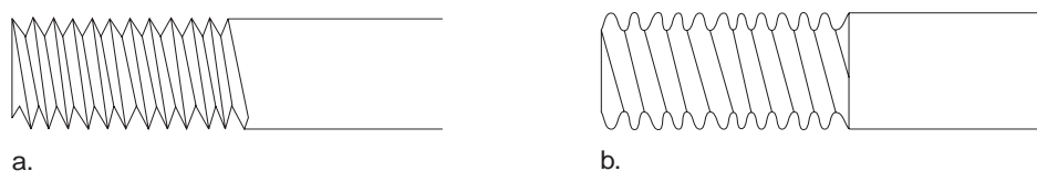
Figure 17.18 Cut threads (a) concentrate stress in the sharp grooves. Rolled threads (b) spread out stresses more evenly.
