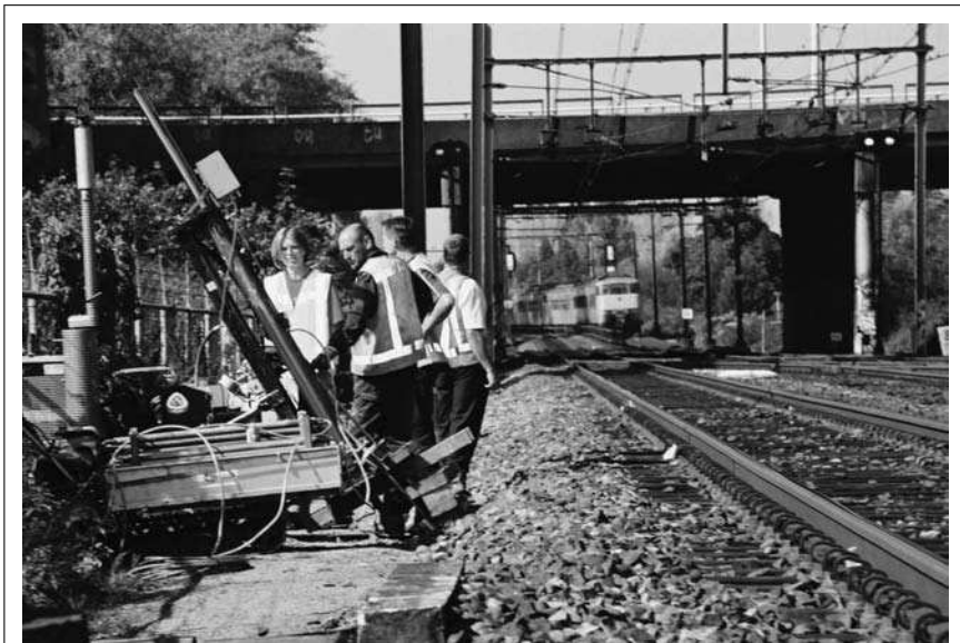
Figure 10.4: In-situ and inclined electrical density testing below a railway (© with permission of GeoDelft).
